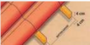
Fig. : 1 Typical dimensions of the tile support element (timber battens). The batten gauge may vary.
