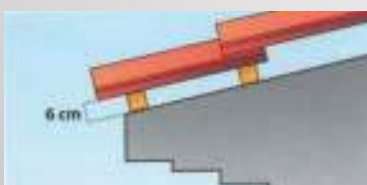
Fig. 4 To maintain the same pitch as the rest of the roof covering, the tiles of the first course should be placed on battens that are two centimetres higher than the others.
