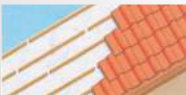
Fig. : 2 The tile supports (battens or mortar fillets) must be laid parallel to the eaves course with gaps of 3-4 cm every 3-4 metres.
